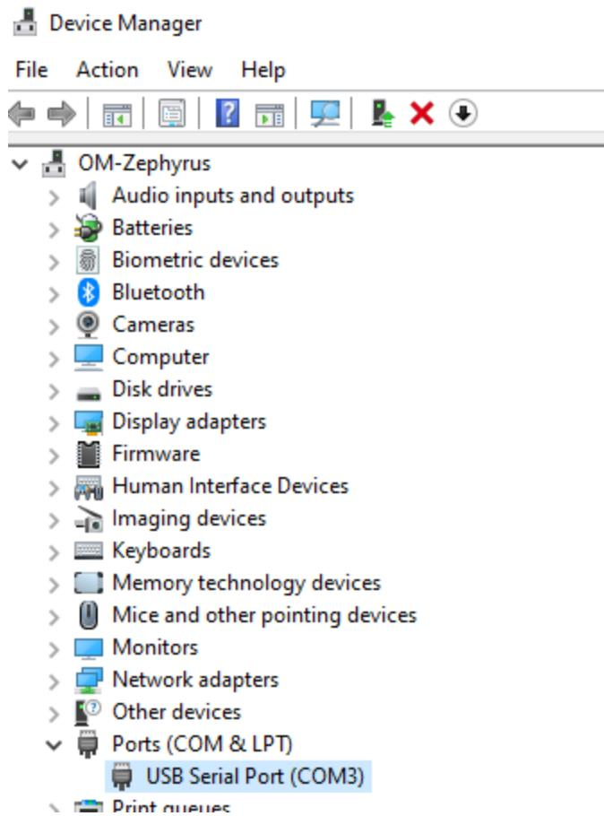
If you are unsure on which device is which, right click on a detected 'USB Serial Port (COMx)' device and choose 'Properties'. On the Properties window that opens, go to the 'Details' tab. Firefly will display as 'Firefly - QRNG PCIe card when selecting the Bus reported device description property.
